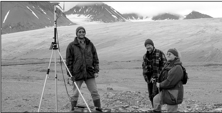
Photo 1.15. GPS-Leica system 500 measurements on the Renardbreen forefield (Photo K. Pękała 2005).
