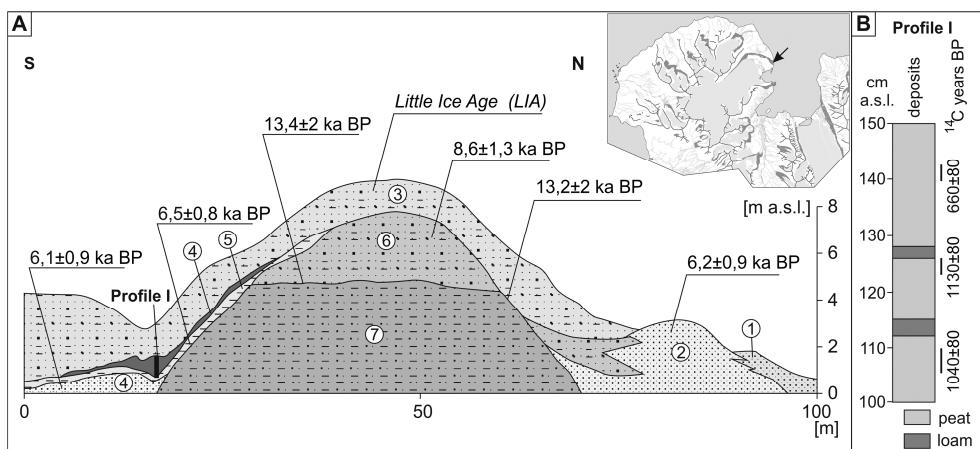
Fig. 2.2.5. A - the geological cross-section of frontal moraine of the Renardbreen (Pękala & Repelewska-Pękalowa 1990): 1- present storm ridge 2- fossil storm ridge, 3- glacial till (Little Ice Age), 4- pushed occupation level of whale settlement with fossil flora (profile 1), 5- clay, 6- glacial till, 7- glacio-marine deposits; B- profile of organic sediments of the Renardbreen-1 site (Dzierżek *et al.* 1990a).
