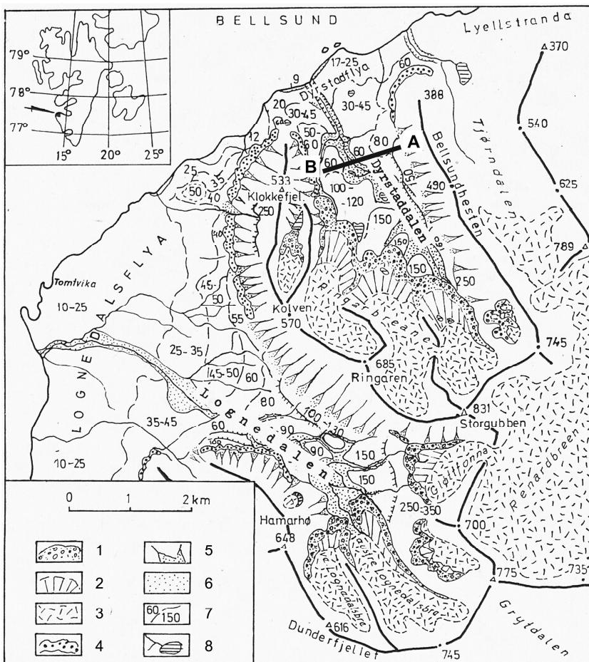
Fig. 2.2.1. Geomorphological map of the Dyrstaddalen and Lognedalen (Pękala & Reder 1989): 1- terminal moraines, 2- ground and ablation moraines, 3- glaciers, 4- nival moraines and rock glaciers, 5- talus fans, 6- outwash plains, 7- marine terraces and denudation levels, 8- streams and lakes; A-B- cross section (see: Fig. 2.2.2).
