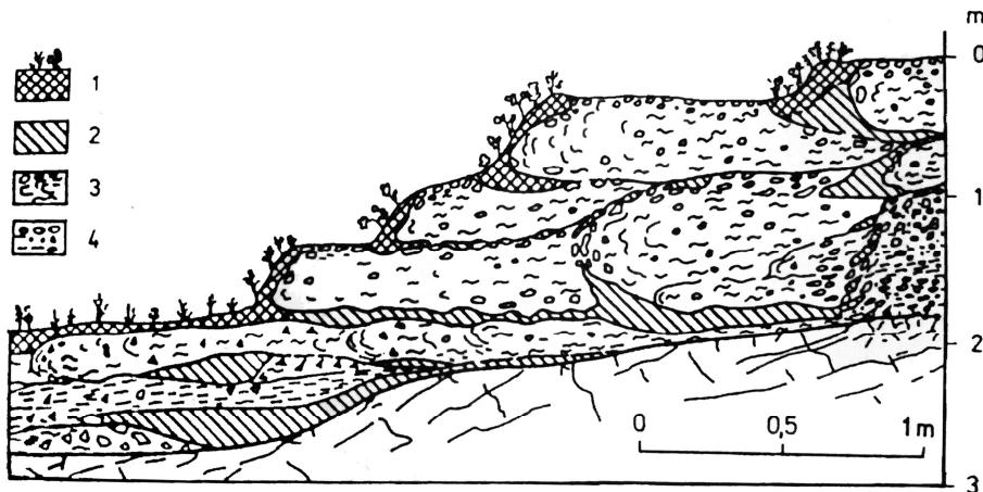
Fig. 2.2.7. Fagerbukta region – garland terrace: 1- vegetation cover and recent soil, 2- peat and fossil soil, 3- solifluction deposits, 4- marine deposits (Repelewska-Pękalowa & Pękala 1993).
